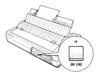
Note: To clear a paper jam, it is recommended **that** you set the printer off line and **use** the **FORM FEED** or **LINE FEED** button. If it is necessary to use the platen knob to clear the jam, be sure to turn the printer off first.
